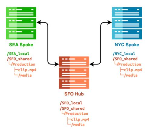
The Cloud Data Fabric functionality lets you make the data on the central cluster available to the remote clusters without the need to replicate data to each location. The data remains available to the edge clusters even if their capacity is lower than that of the central cluster. While a read-write portal lets the edge clusters create or modify data on the central cluster, a read-only portal lets only the edge clusters read data from the central cluster.
