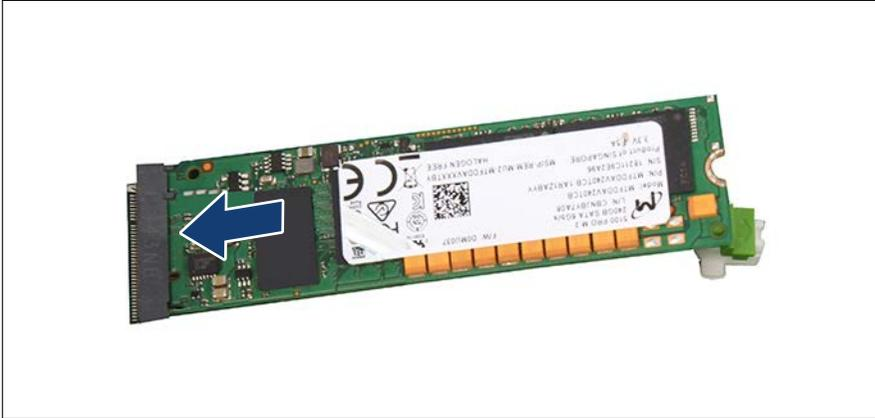
Figure 107: Installing the M.2 SSD (A)
