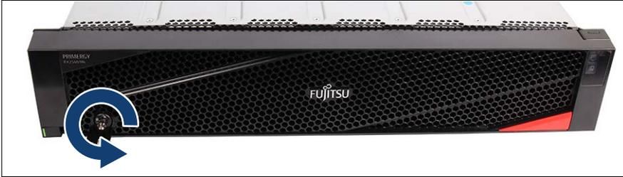
Figure 23: Turning the key
