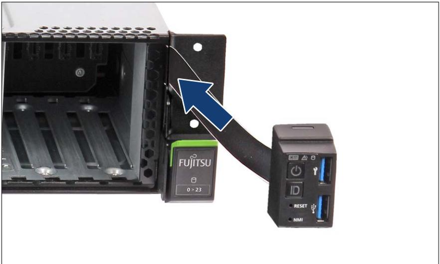
Figure 320: Installing the COP (B)
