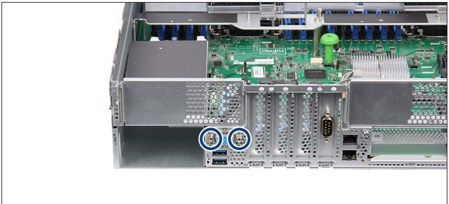
Figure 337: Installing the rear VGA connector (B)
