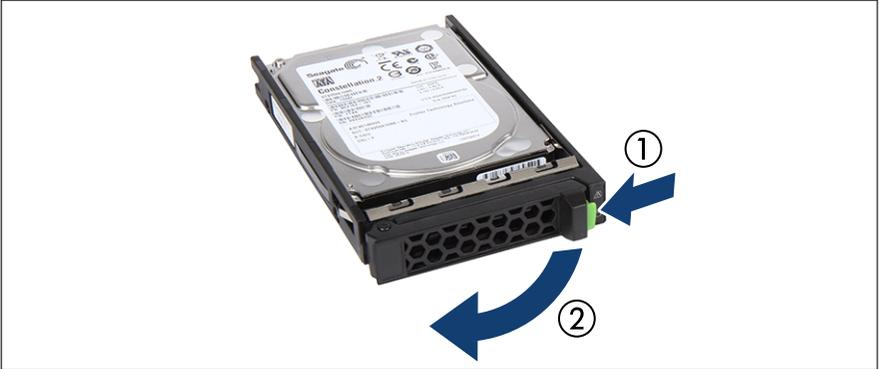
Figure 85: Opening the locking lever
