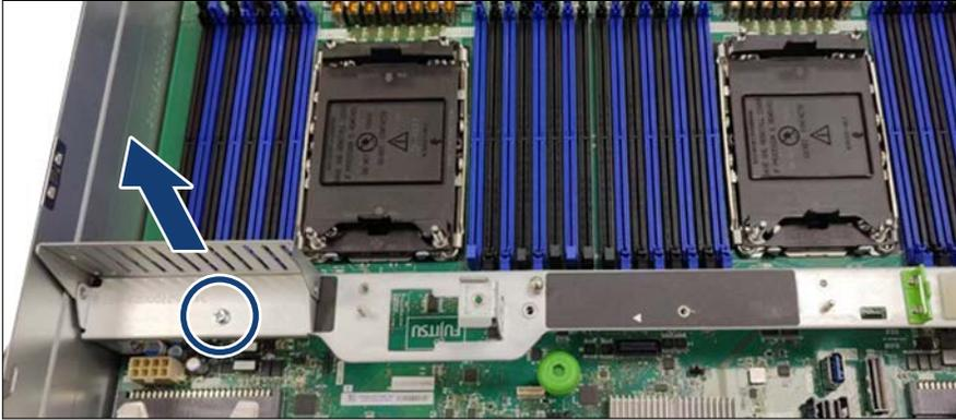
Figure 162: Removing the GPU dummy bracket
