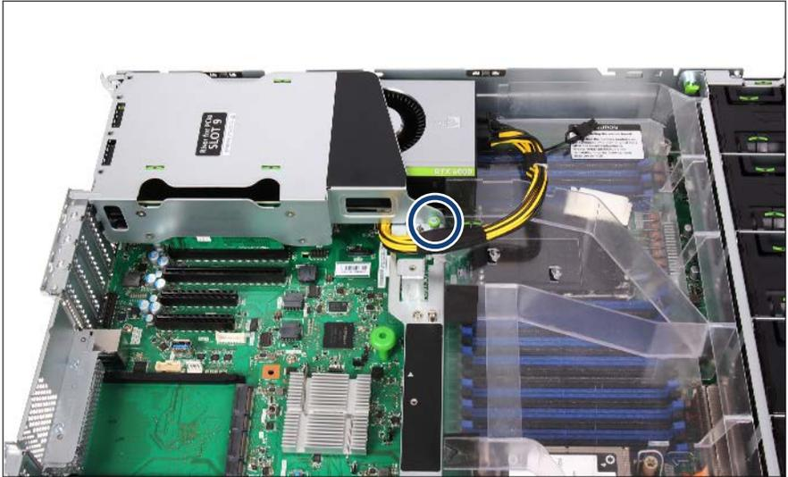
Figure 27: Installing the riser module 2
