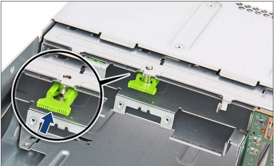
Figure 300: Installing the RDX drive (C)
