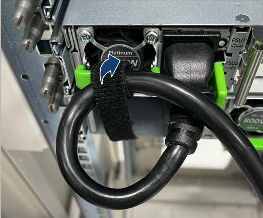
Figure 5: Loosening the hook-and-loop tape
