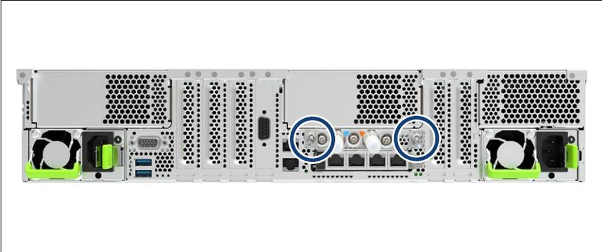
Figure 237: Removing the screws
