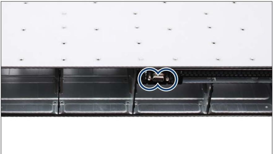
Figure 324: Installing the front VGA
