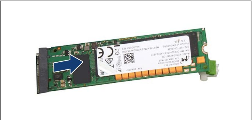
Figure 110: Removing the M.2 SSD (B)
