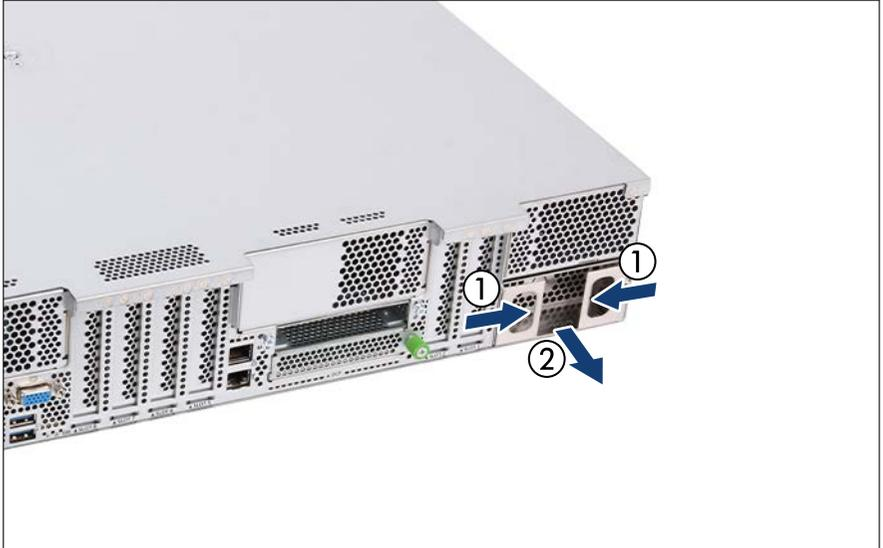
Figure 46: Removing the dummy cover
