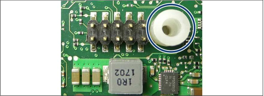
Figure 342: Inserting the TPM spacer on the system board
