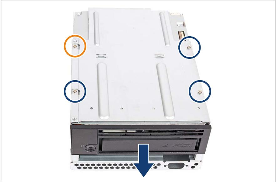
Figure 289: Removing the LTO drive (C)
