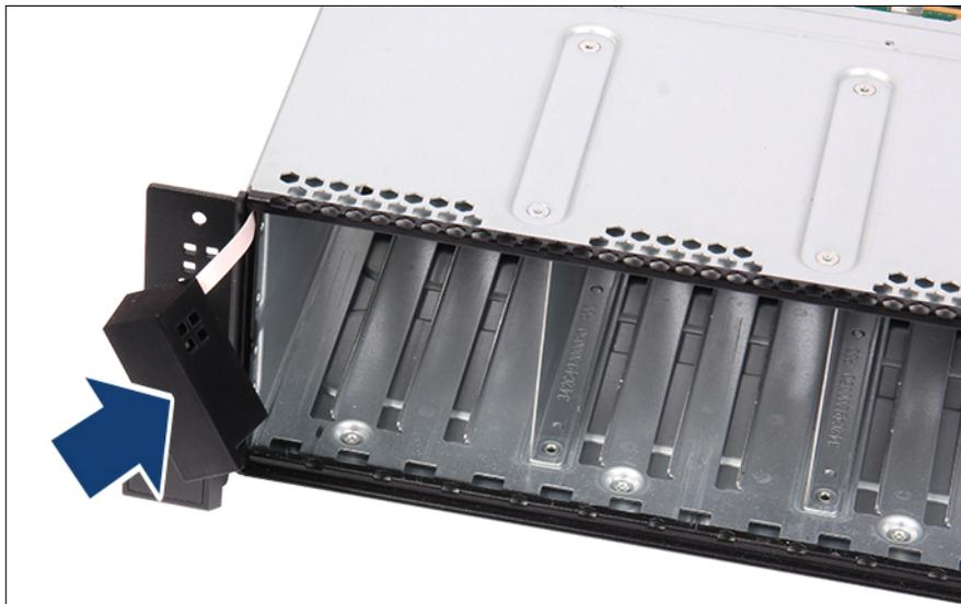
Figure 314: Installing the thermal sensor
