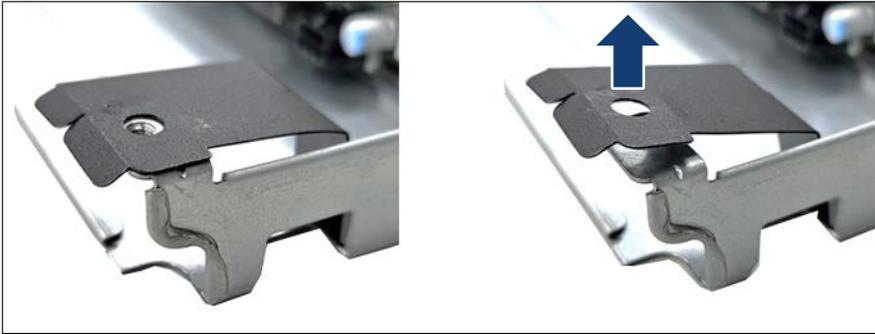
Figure 170: Moving the Mylar foil (A)
