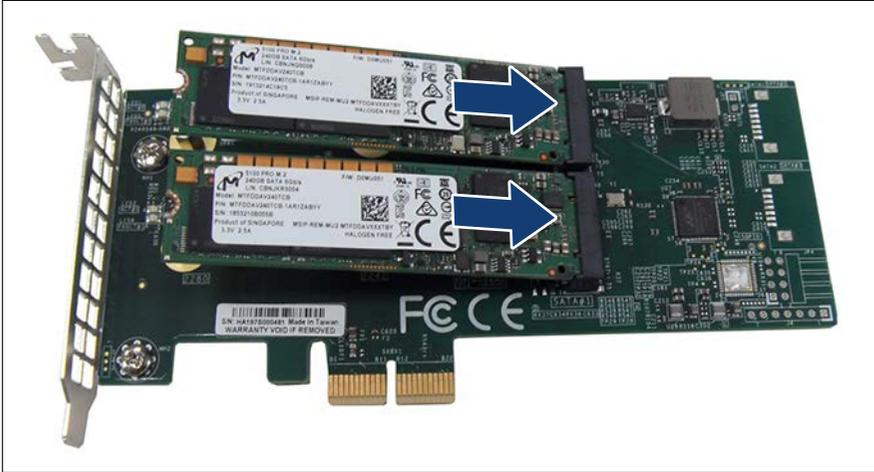
Figure 155: Installing M.2 SSDs (A)
