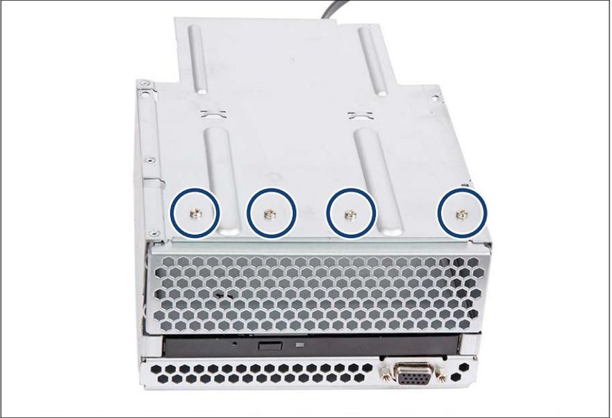
Figure 280: Removing the air grid (A)
