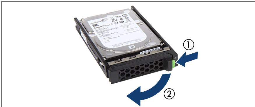
Figure 87: Opening the locking lever
