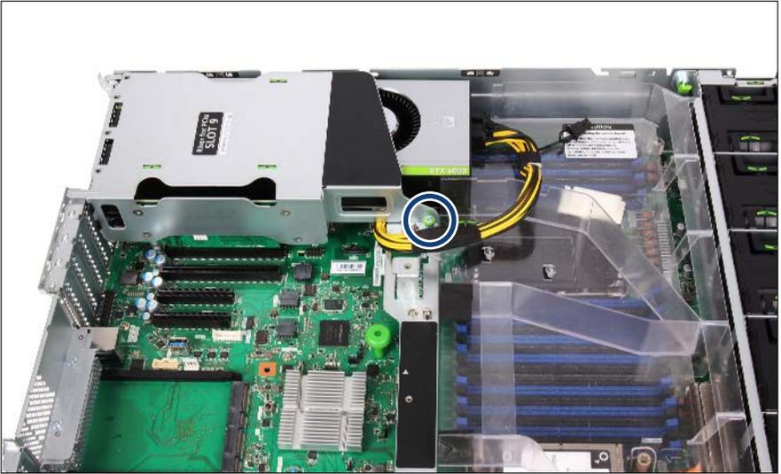
Figure 25: Removing the riser module 2
