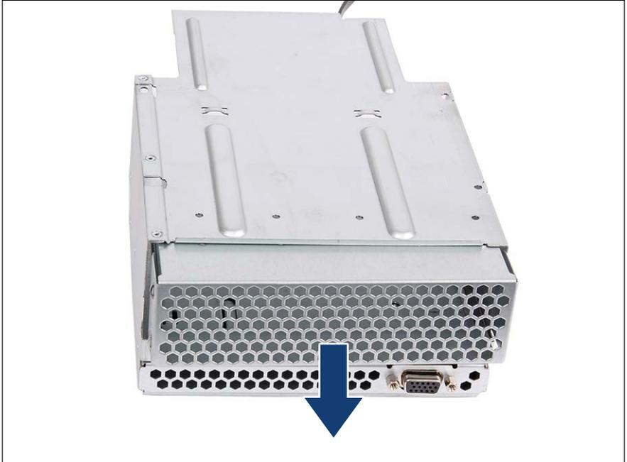
Figure 297: Removing the air grid (B)
