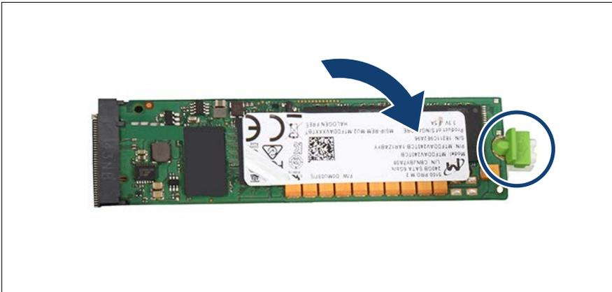
Figure 108: Installing the M.2 SSD (B)
