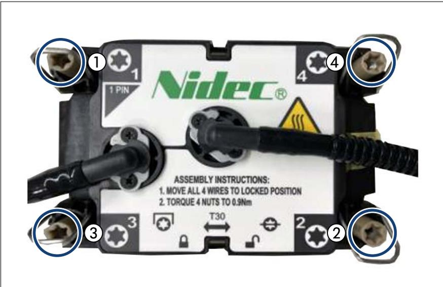
Figure 238: Removing the LC heat sink (A)
