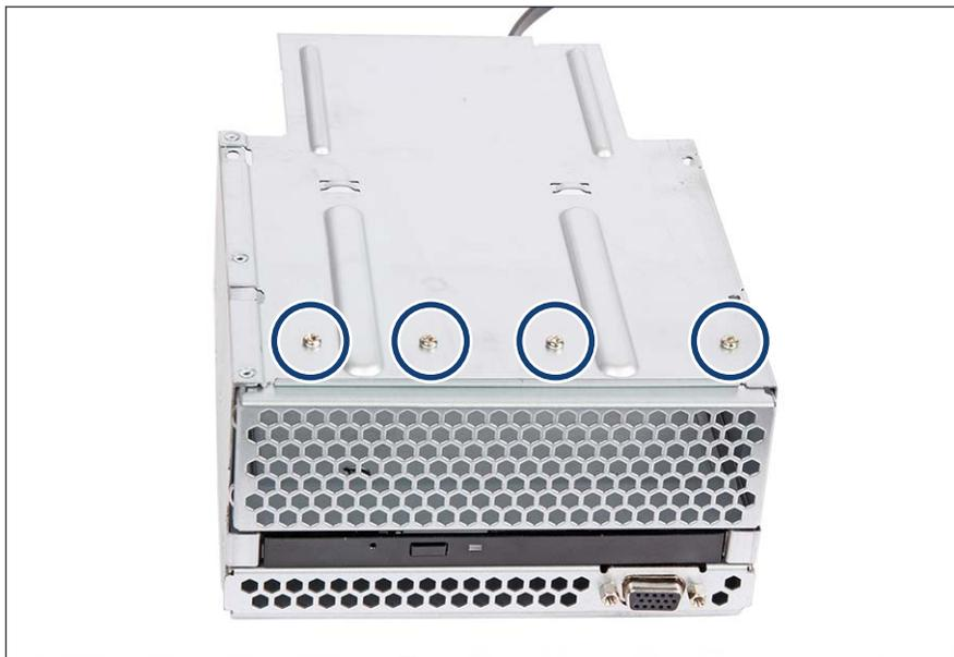
Figure 296: Removing the air grid (A)
