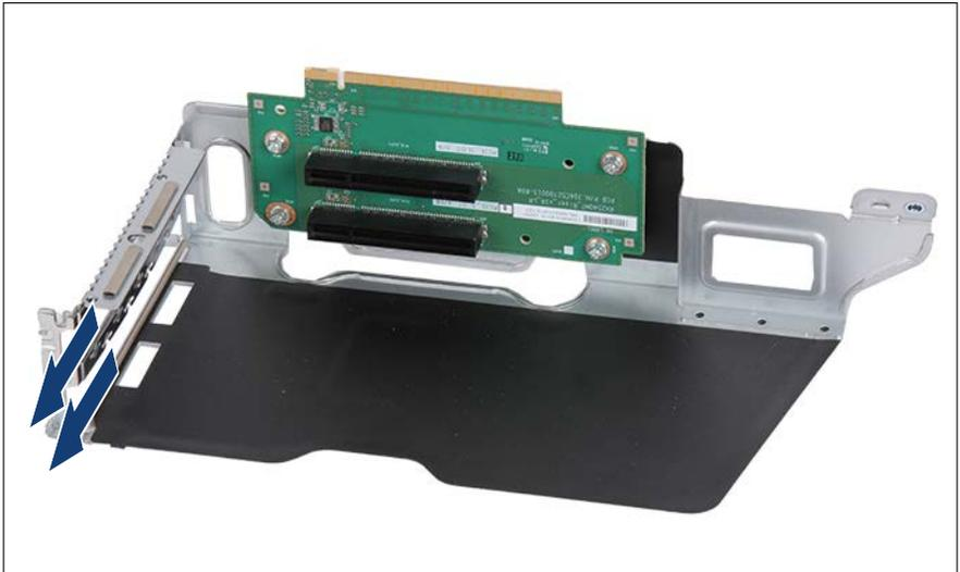
Figure 184: Removing the two slot covers
