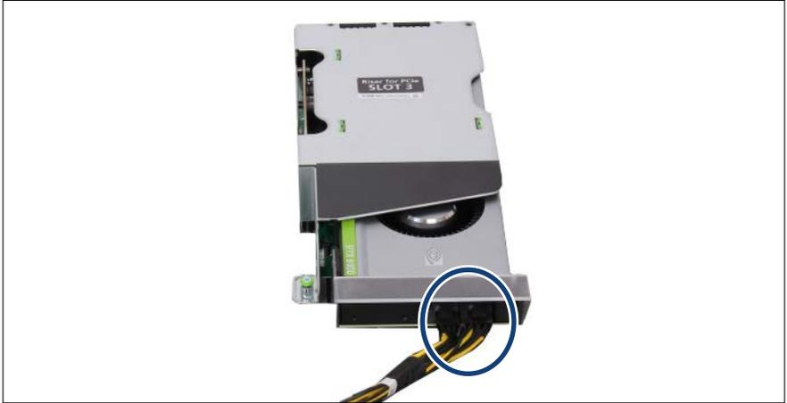
Figure 160: Connecting the GPU power cable
