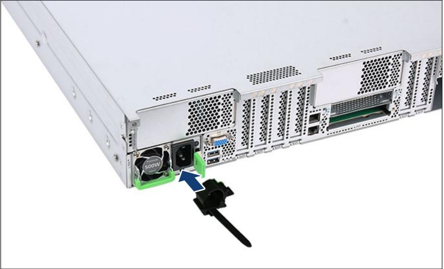
Figure 48: Installing the cable clamp
