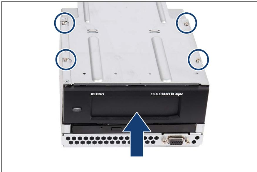
Figure 298: Installing the RDX drive (A)
