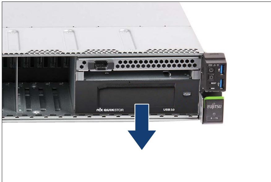
Figure 304: Removing the RDX drive (B)
