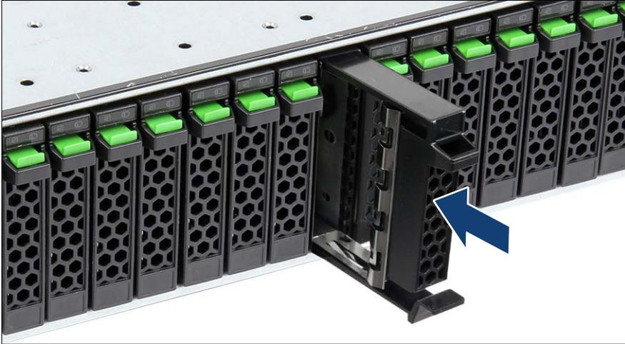
Figure 88: Installing the 2.5-inch HDD/SSD dummy module
