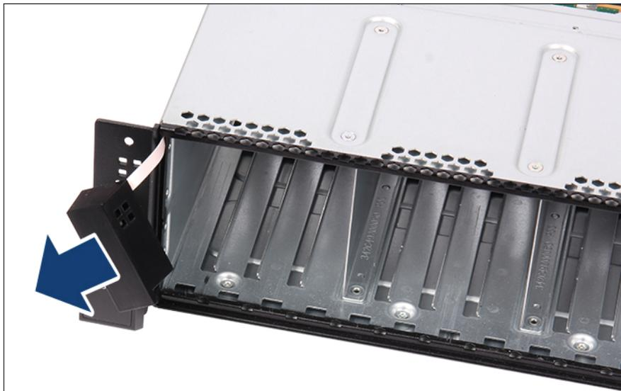
Figure 312: Removing the thermal sensor
