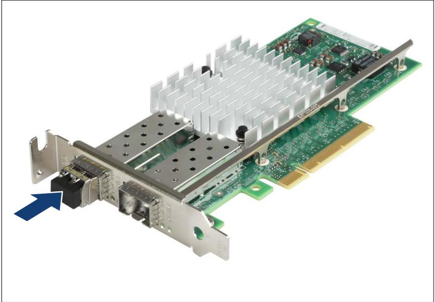
Figure 137: Installing the protective cap
