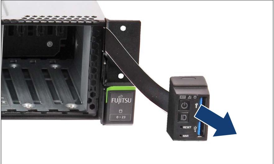
Figure 319: Removing the COP (B)
