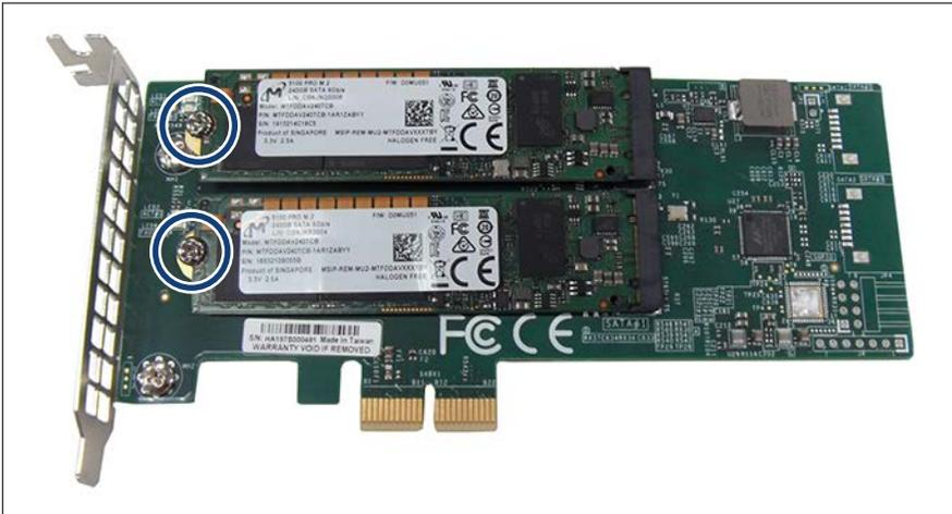
Figure 156: Installing M.2 SSDs (B)
