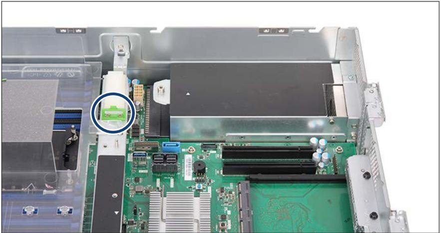
Figure 252: Storing the ODD latch
