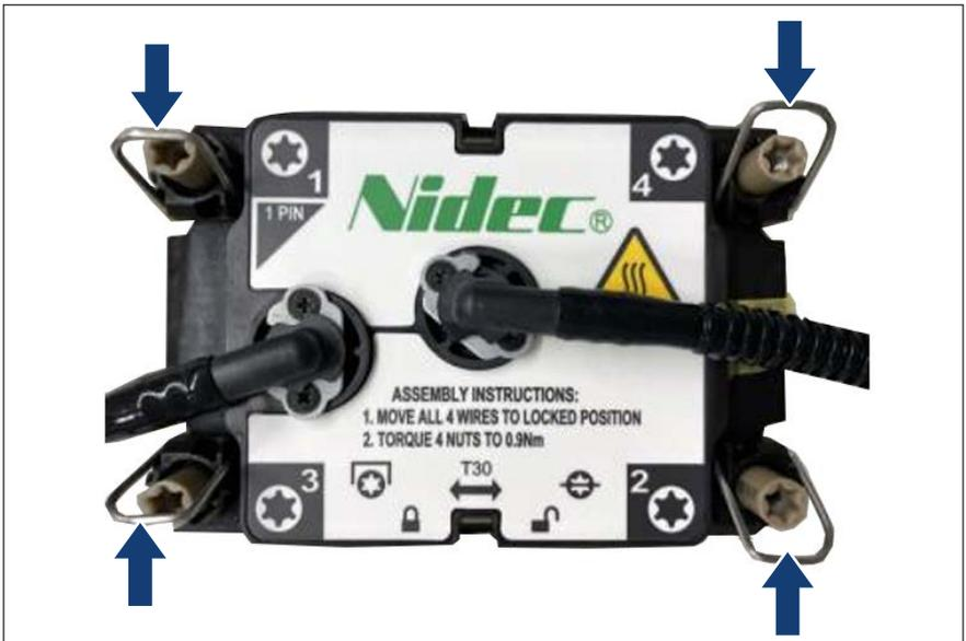
Figure 239: Removing the LC heat sink (B)
