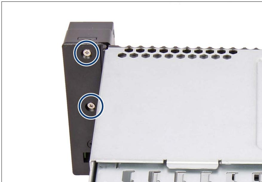
Figure 318: Removing the COP (A)
