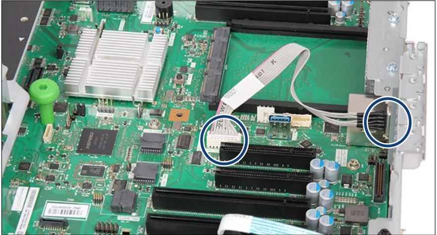
Figure 332: Disconnecting the serial interface
