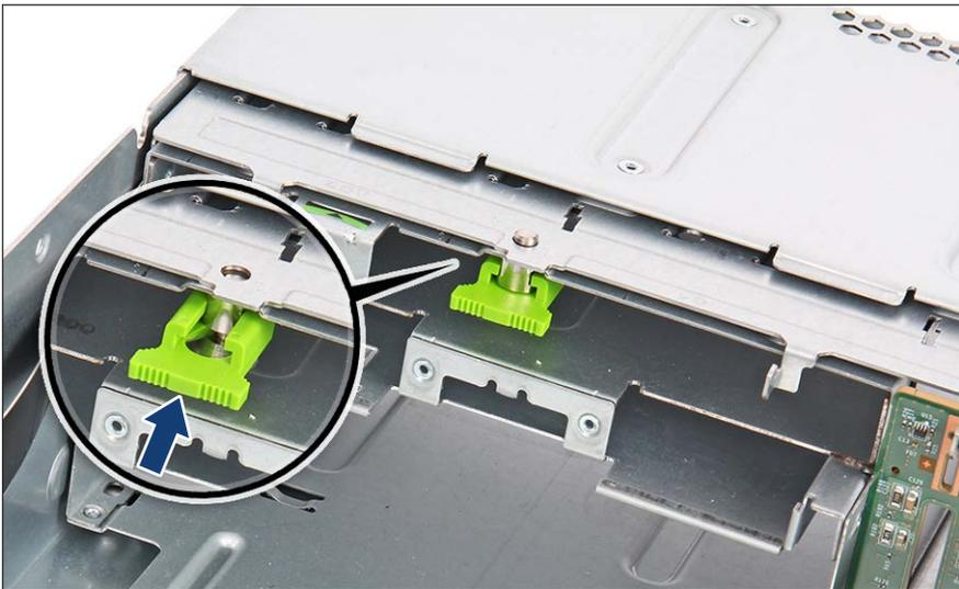
Figure 284: Installing the LTO drive (C)
