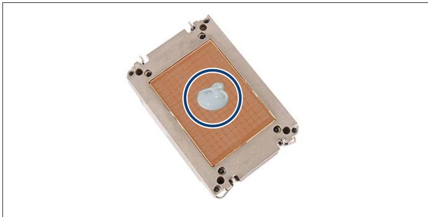
Figure 235: Applying the thermal paste
