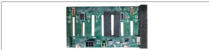
Figure 91: 8x 2.5-inch HDD backplane with two foams
