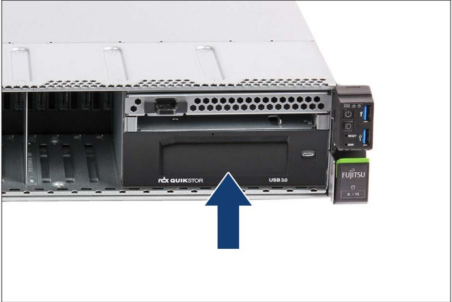
Figure 299: Installing the RDX drive (B)
