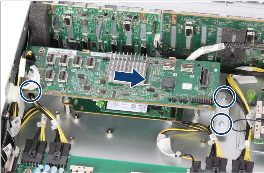
Figure 104: Removing the SAS expander board holder
