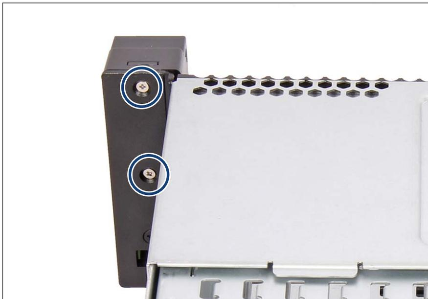
Figure 321: Installing the COP (B)
