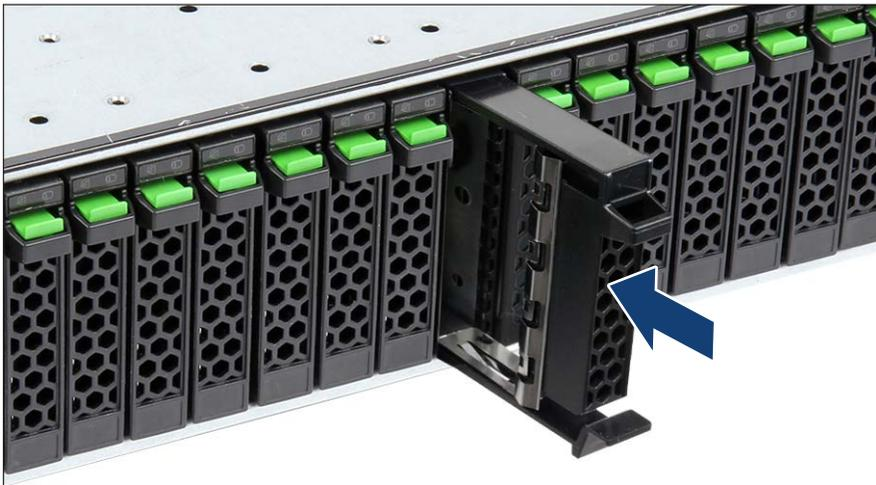
Figure 82: Installing the 2.5-inch HDD/SSD dummy module
