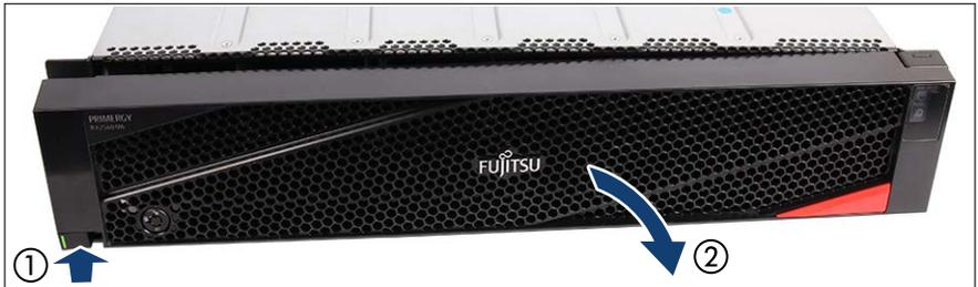
Figure 3: Removing the front cover
