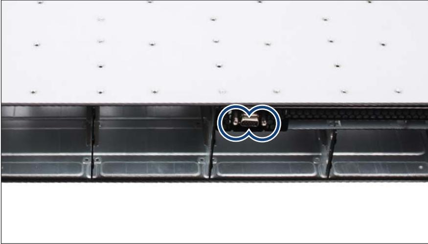
Figure 326: Removing the front VGA
