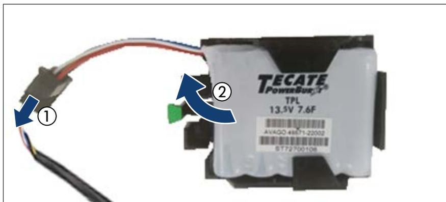
Figure 198: Removing the FBU from the holder
