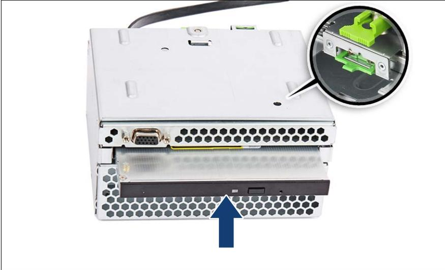
Figure 255: Installing the ODD
