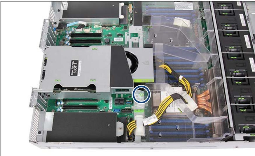
Figure 24: Removing the riser module 1
