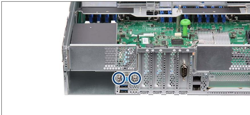
Figure 334: Removing the rear VGA connector (A)
