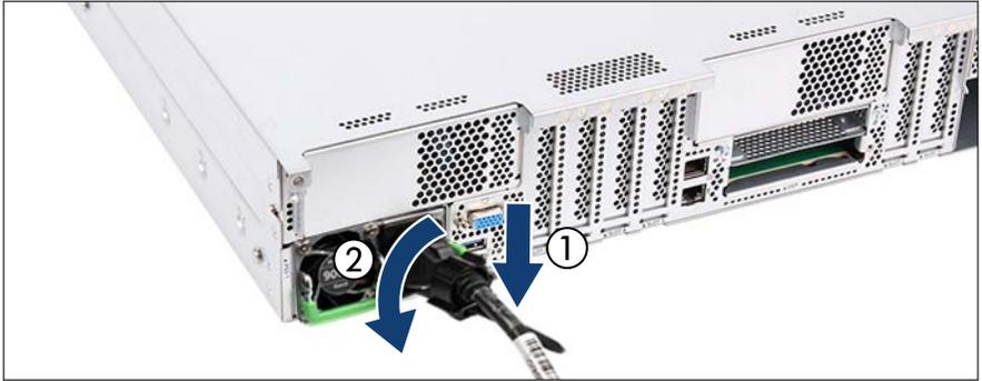
Figure 4: Unlocking the cable clamp of a PSU
