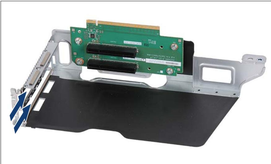
Figure 187: Installing the two slot covers
