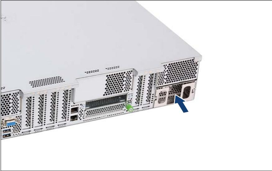
Figure 51: Installing the dummy cover
