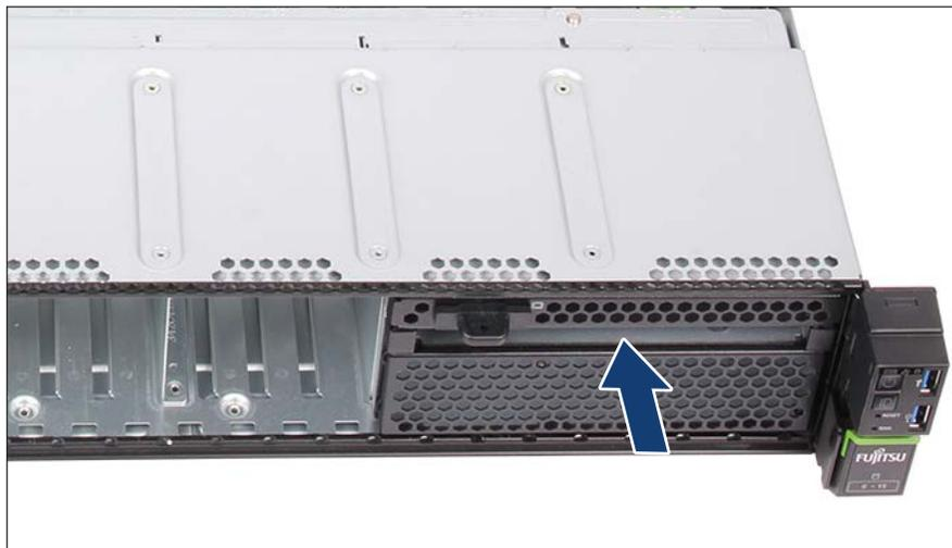
Figure 261: Installing the dummy cover
