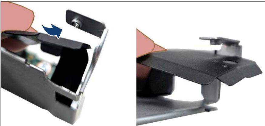
Figure 171: Moving the Mylar foil (B)
