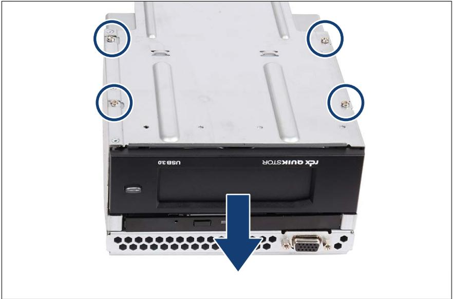
Figure 305: Removing the RDX drive (C)
