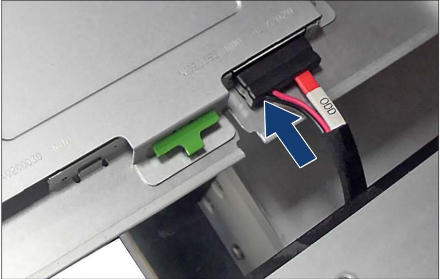
Figure 266: Connecting the ODD cable
