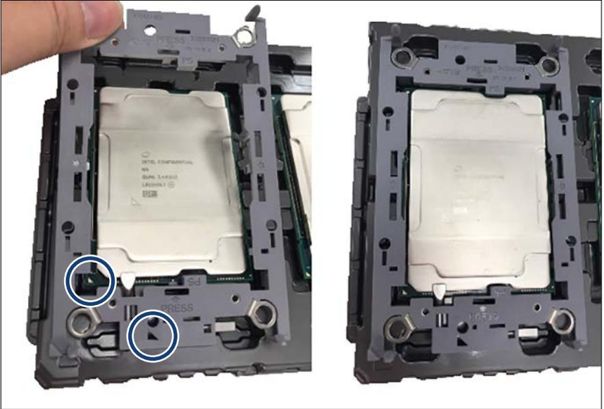
Figure 221: Installing the CPU frame on the CPU
