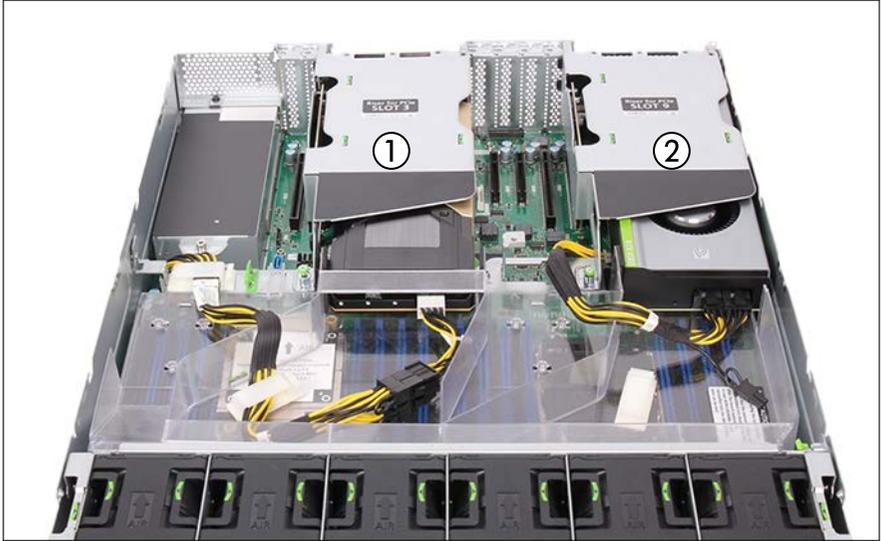
Figure 129: Positions of riser modules
