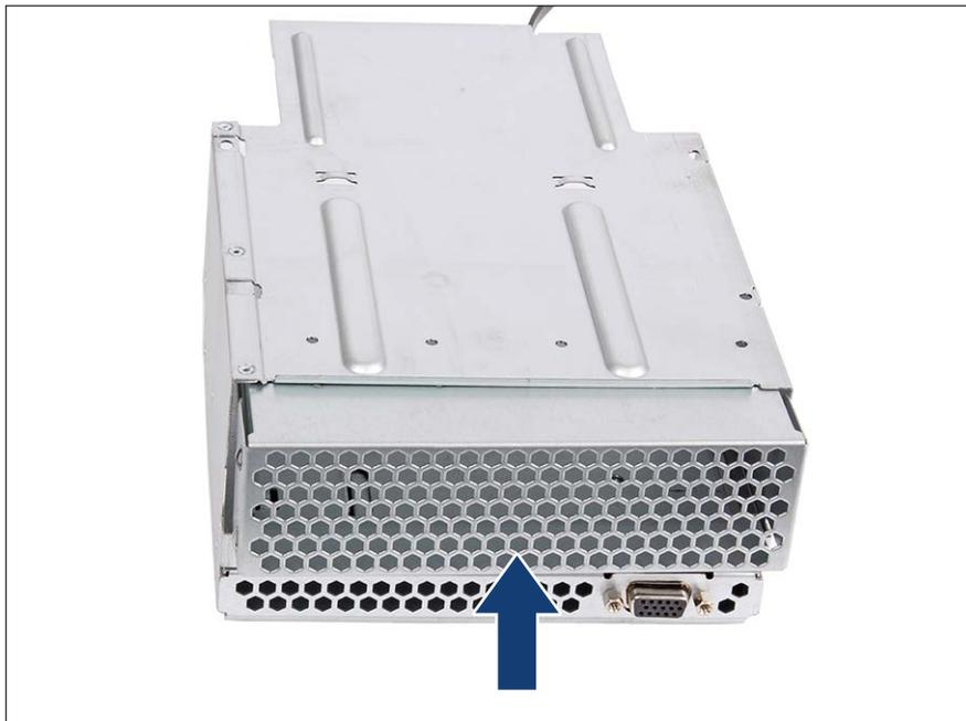
Figure 306: Installing the air grid (A)
