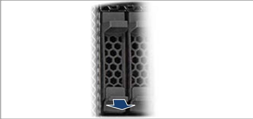
Figure 83: Removing the dummy lock
