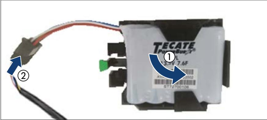
Figure 194: Installing the FBU in the holder
