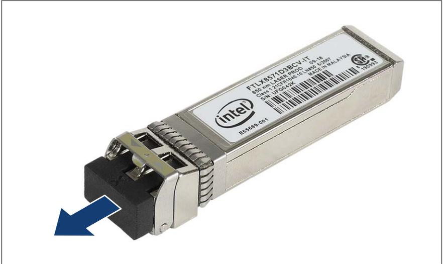
Figure 133: Removing the protective cap
