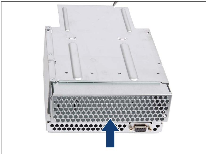
Figure 290: Installing the air grid (A)
